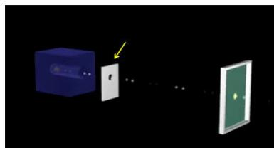
Further research by Becquerel, Ernest Rutherford, Madam Curie, and others discovered 3 types of radiation. Here's how they did it. A radiation source shines on a lead plate with a small hole in it to create a beam. The beam is directed at a fluorescent screen. The screen flashes when it is struck.
