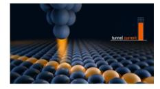
It has a small pin head that is actually one single atom at its tip. The tip is brought close enough to the object for electrons to tunnel across the space exactly in accordance with Schrodinger's equation. This creates an electric current.
