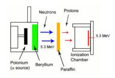
The key was working energy considerations back from the protons ejected from the paraffin on the right to the energy required in the radiation coming out of the Beryllium on the left. The conclusion was that the particles hitting the paraffin were of the same mass and energy as the protons but without any charge. At this point it was generally accepted that the neutron had indeed been discovered.
