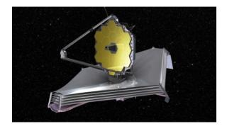
To help find solutions to problems like these, the next generation space telescope is in development. Scheduled for launch in 2018, the James Webb Space Telescope is optimized for observations in the infrared, and a scientific successor to the Hubble Space Telescope and the Spitzer Space Telescope. It will be almost three times the size of Hubble, and orbit far from Earth in the Earth—Sun L<sub>2</sub> Lagrange point.
