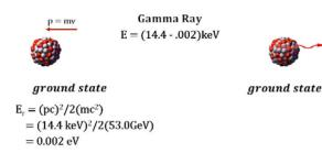
What Mossbauer discovered was that if he imbeds the atoms in a crystal, the recoil is reduced dramatically, and absorption can be established.
