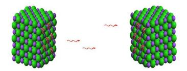
Pound and Rebka use this Mossbauer Effect. They placed an emitter at the bottom of a tower in the Laboratory and installed a detector 22.6 meters above. No absorption was detected because gravitational time dilation changed the frequency of the emitted gamma rays so no energy match existed in the detector.
