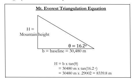
[Additional info: Surveyors have created networks of triangulations that covered entire countries like France, Great Brittan, and India using spherical trigonometry to account for the curvature of the planet. With these networks, we can triangulate everything that can be seen on our planet.
