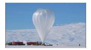
Our knowledge in this area didn't really begin until the late 1700s when high flying balloons came into use. Here's a scientific balloon launch. High altitude balloons have been used for over 70 years for atmospheric exploration. They fly at altitudes in excess of 32 km (20 miles) above the surface of the earth for days on end.
