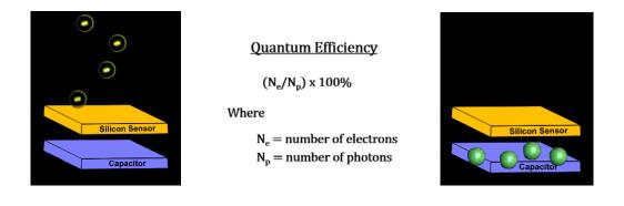
The phonons start producing electrons as soon as the shutter is opened. The capacitor collects the freed electrons until the shutter is closed. At that point, the voltage across the capacitor represents the number of electrons the capacitor collected. This information is sent to the computer.
