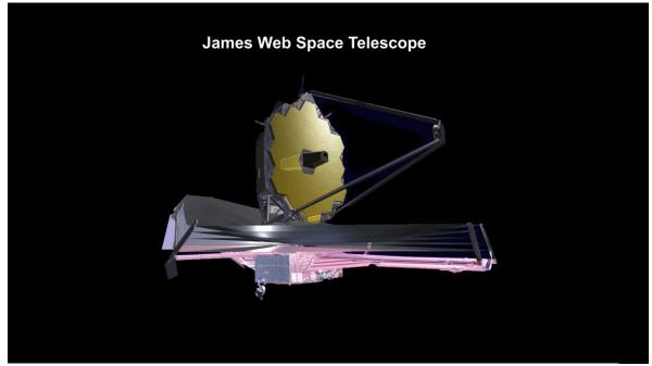
Here are Web's primary and secondary mirrors. The primary is the size of a tennis court. This animation shows the light path through the telescope. The light reflects off the primary and is focused onto the secondary, where it is beamed into the camera. Webb's mirrors are covered in a microscopically thin layer of gold, which optimizes them for reflecting infrared light.
