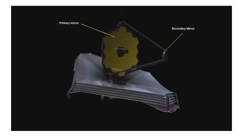
Other key components include the camera, the sunshield, the solar panels, communication antenna, computer, and spacecraft control. The sunshield is particularly important because of the telescope's extreme sensitivity to heat. Webb primarily observes infrared light, which can sometimes be felt as heat. Because the telescope will be observing the very faint infrared signals of very distant objects, it
