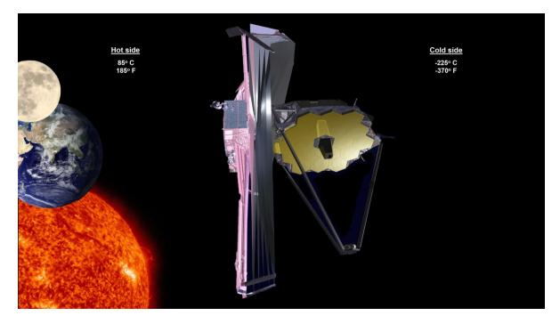
So, to have the sunshield be effective protection against the light and heat of the Sun, Earth and Moon, these bodies all have to be located in the same direction. This is why the telescope must be out at the  $L_2$  Lagrange point 1.5 km from Earth. That's 1 million miles.
