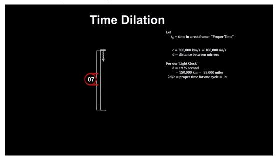
Now if we put the clock into motion with respect to a ground-based observer, we see that the light has to travel further, and because its speed is constant, it will take longer. The moving light clock is therefore running slower than a stationary duplicate. This is called time dilation. It's the geometry of the situation that gives us the conversion factor.
