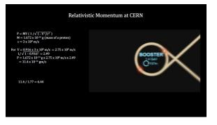
The protons are then flung into the proton synchrotron. They circulate here for 1.2 seconds reaching 99.9 % of the speed of light. At this speed their momentum has increased by more than 60 times [to  $112 \ge 10^{-16} \text{ gm/s}$ ].
