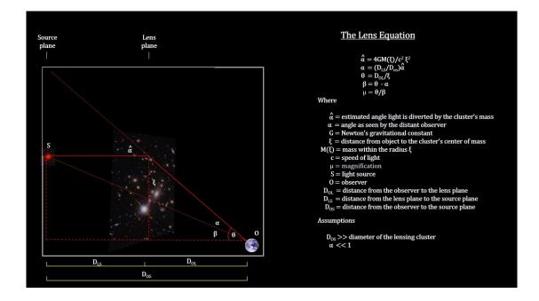
Note that the magnitude of the light bending changes for object's closer to the lens. The lens' magnification will decrease as the ratio of the distance from the lens to the object over the distance of the lens to the observer decreases.
